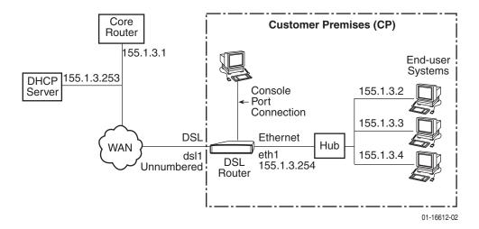
In this DHCP Relay with Proxy ARP example:
